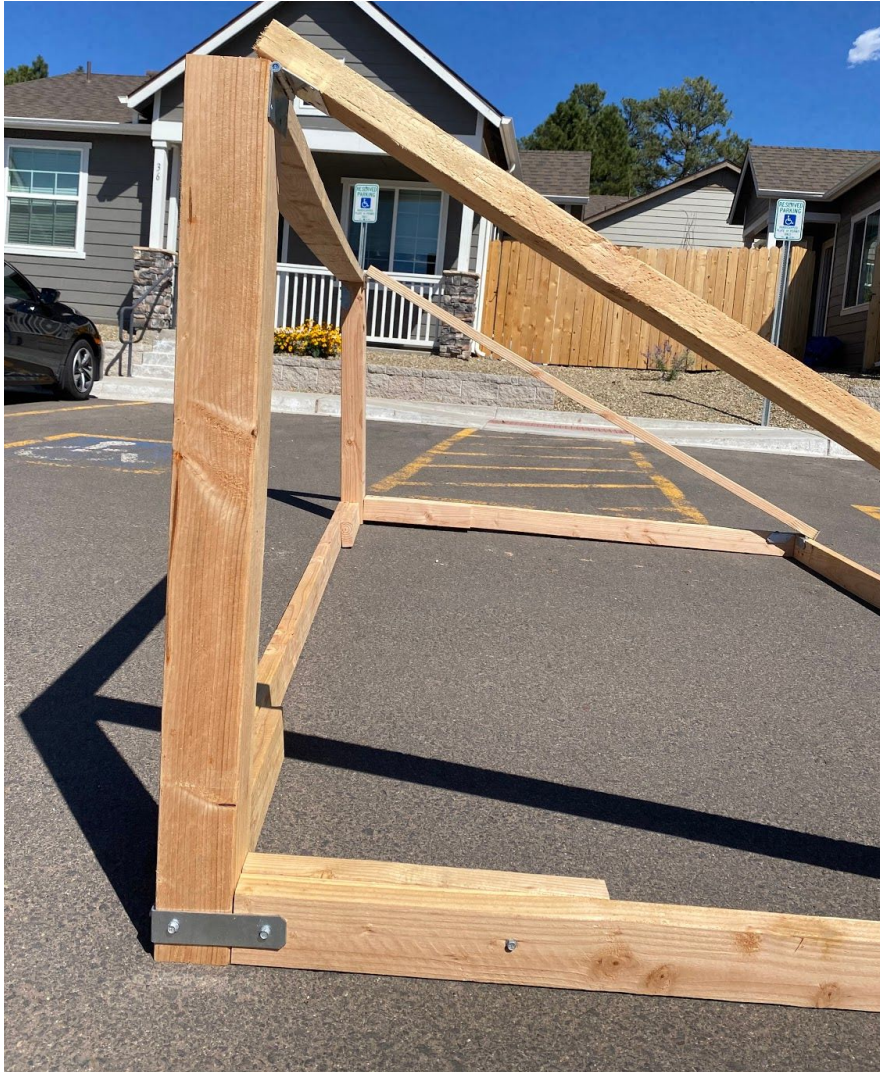
Figure 3: Load-bearing 90 degree angle joint
